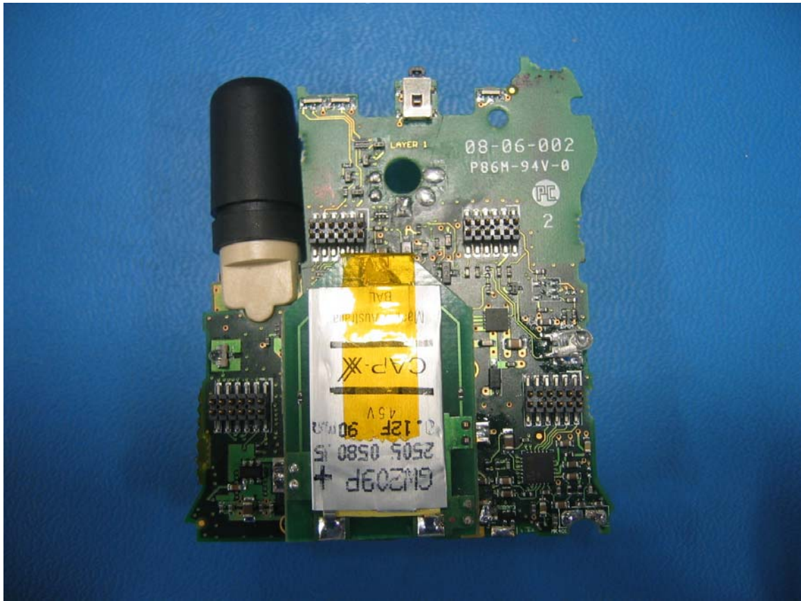
SIM PCB with supercap
