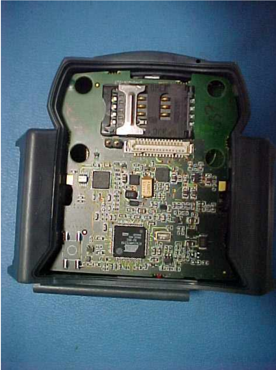
Antenna & SIM in main shell
