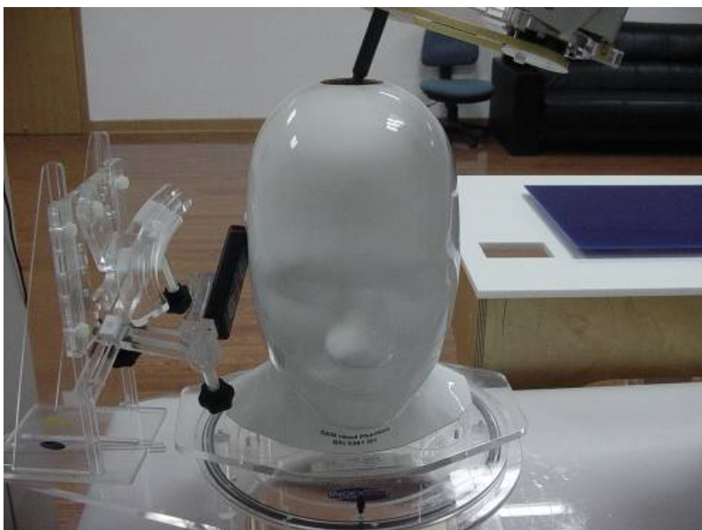
Fig.6 EUT Right Head Tilt15 Position
