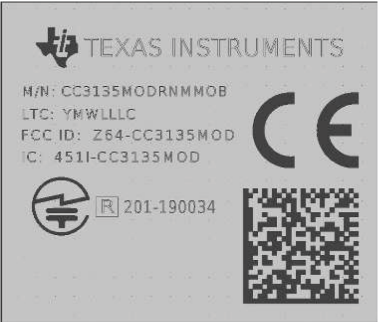
Figure 8-1. SimpleLink™ CC3135 Module Markings
