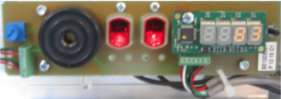
Figure 4.4: Light Barrier Latest assembly with 4 LED 7-segment Displays (latest model)
