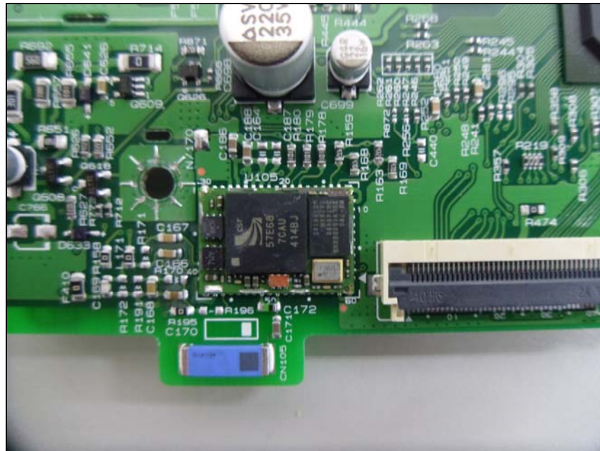
Top view of Module and Chip Antenna
