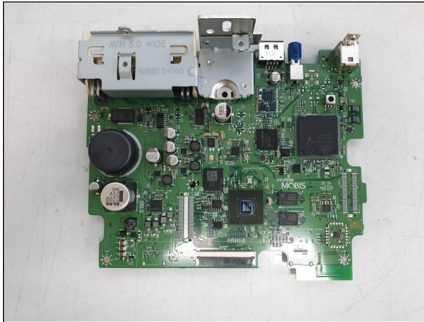
Bottom view of Main PCB
