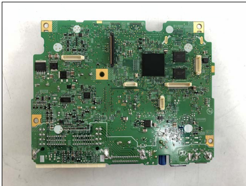
Bottom view of Main PCB
