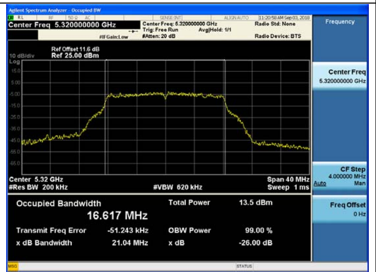
802.11a UNII 3 BAND 26dB Bandwidth (CH 157)
