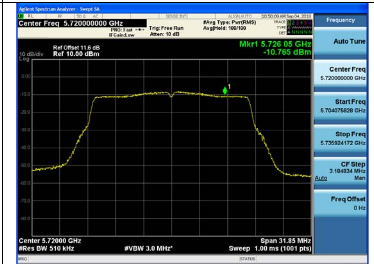
802.11n_HT20 UNII 3 Band PSD CH.144
