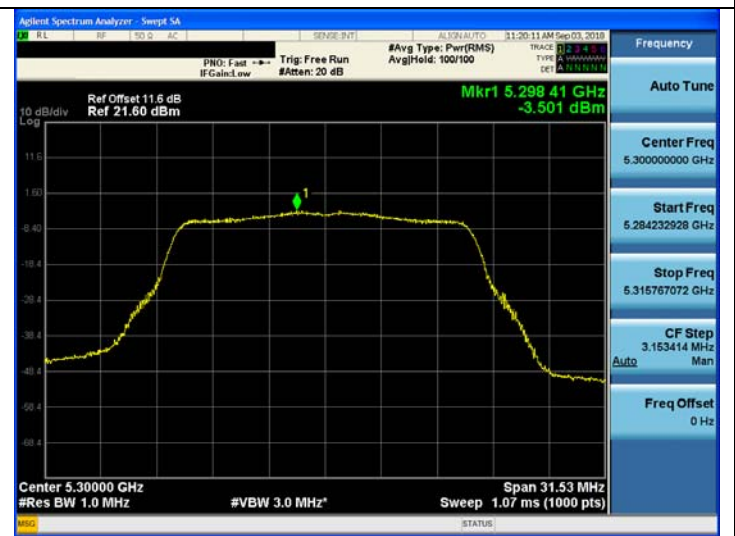
802.11a UNII 3 BAND PSD CH 157
