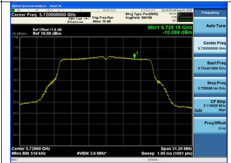
802.11n_HT20 UNII 3 Band PSD CH.144
