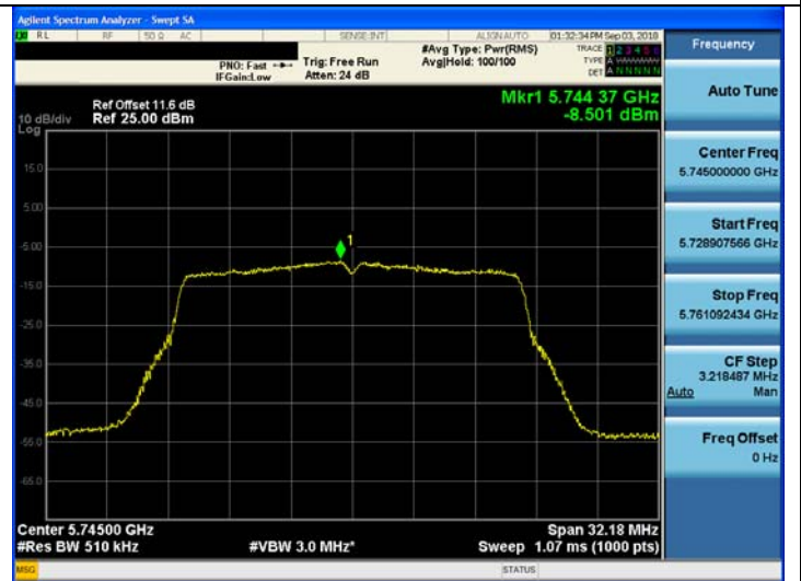
802.11n_HT20 UNII 3 BAND PSD CH 149
