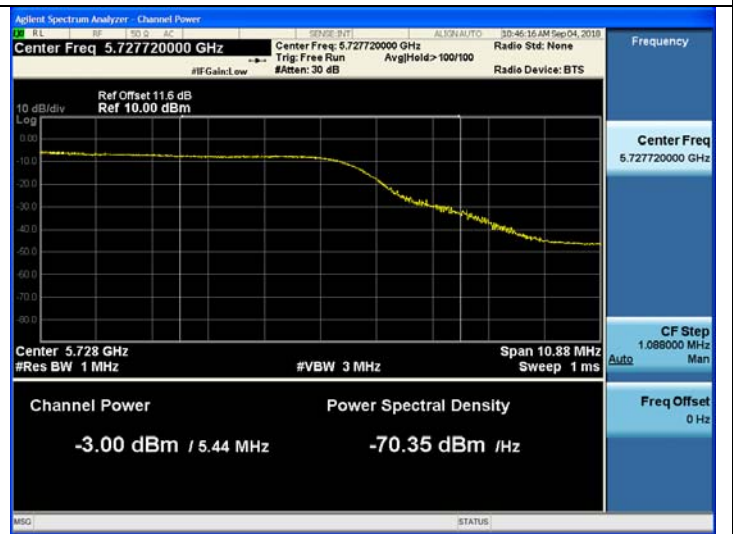
802.11n_HT20 UNII 3 Band Average Power CH.144
