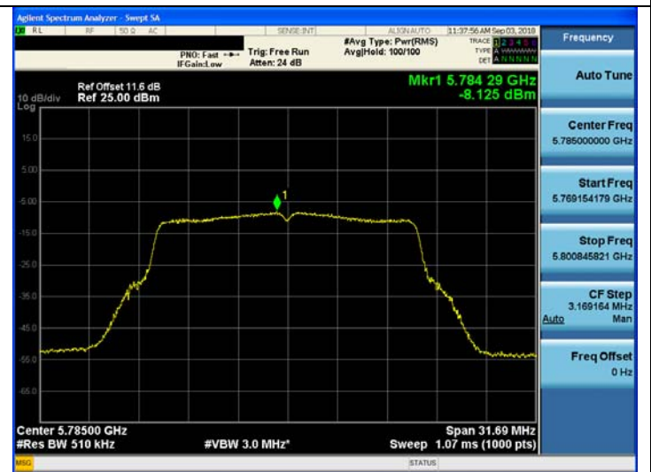
802.11a UNII 3 BAND PSD CH 157
