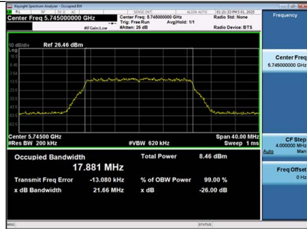
802.11n(HT40) 26 dB Bandwidth (CH 38)
