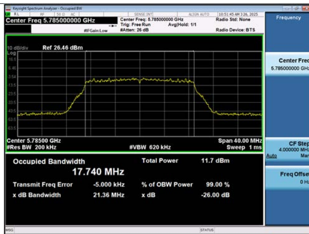
802.11ac(VHT40) 26 dB Bandwidth (CH 159)
