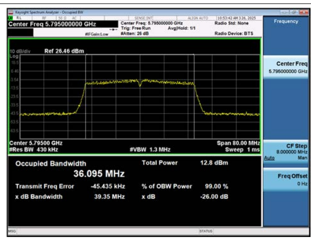
802.11ac(VHT80) 26 dB Bandwidth (CH 42)
