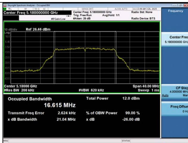
802.11ac(VHT20) 26 dB Bandwidth (CH 157)
