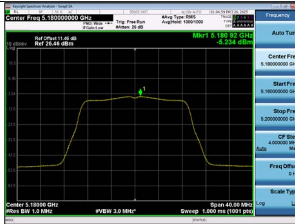
Bandwidth 40M, 802.11ac(VHT40) (Ch. 46)
