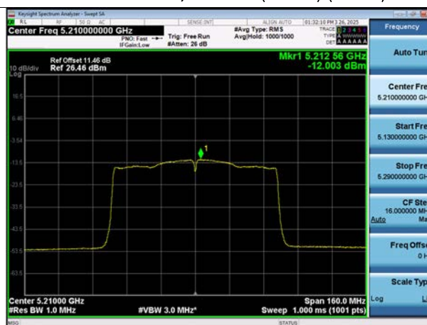
Bandwidth 80M, 802.11ac(VHT80) (Ch. 42)
