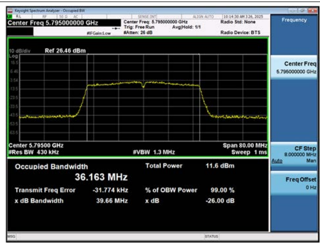
802.11ac(VHT80) 26 dB Bandwidth (CH 155)
