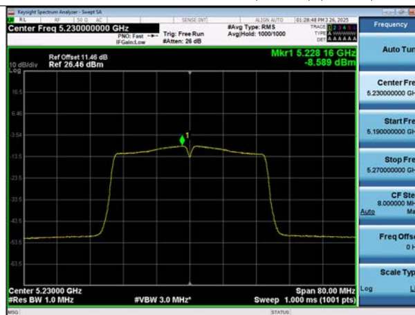
Bandwidth 80M, 802.11ac(VHT80) (Ch. 42)
