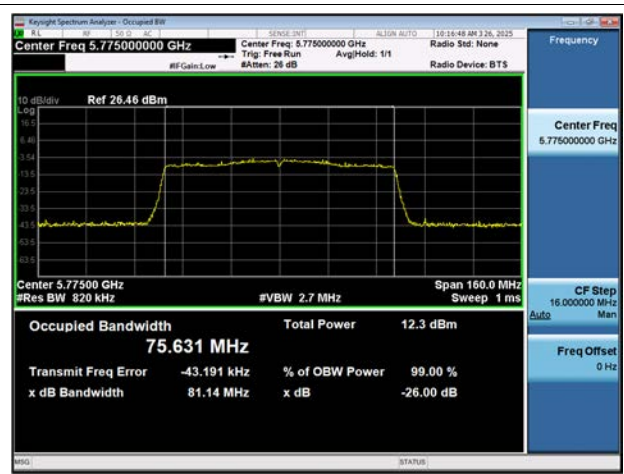
802.11ac(VHT80) 26 dB Bandwidth (CH 155)
