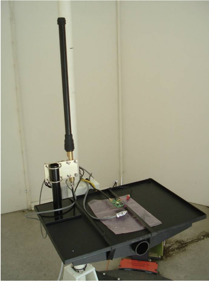
Radiated Emissions Test Setup
