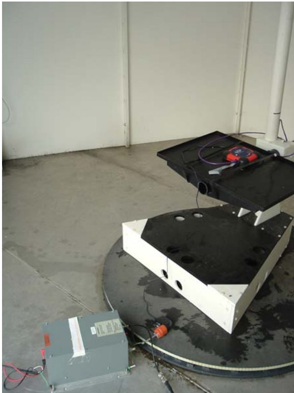
Conducted emissions test setup
