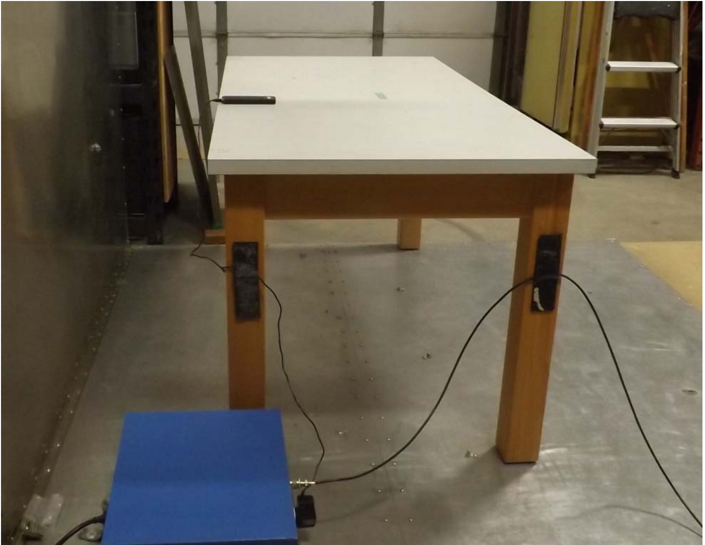
Figure E23.2 – Setup – AC Line Conducted
