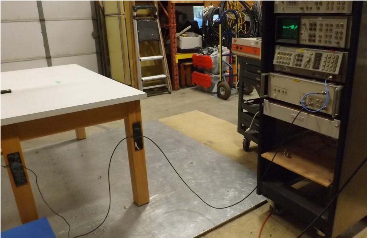
Figure E23.4 – Setup – AC Line Conducted
