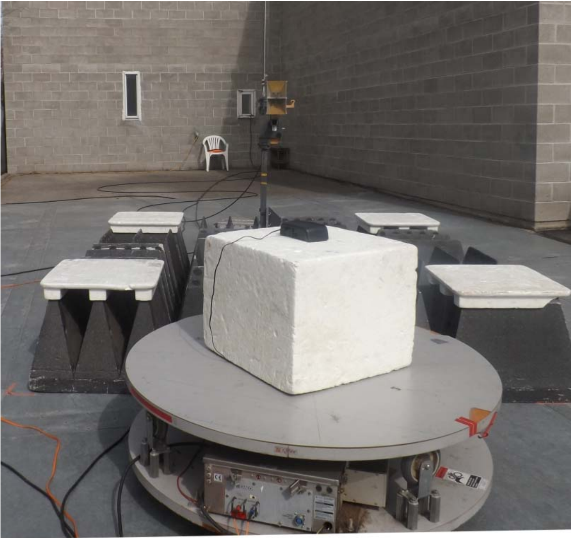
Figure E14.4 – Setup – Radiated Emissions 1 - 18GHz, Horizontal
