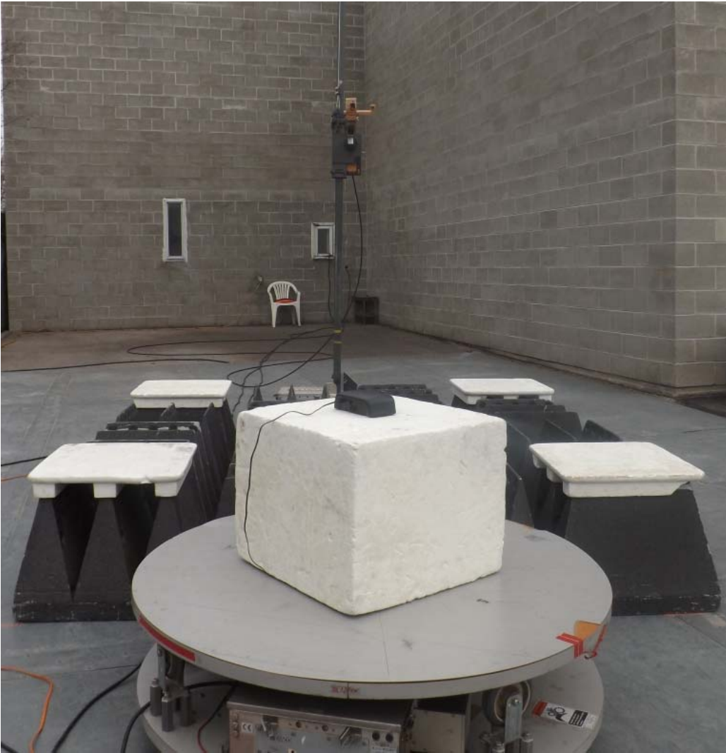
Figure E14.6 – Setup – Radiated Emissions 18 – 26.5GHz, Horizontal
