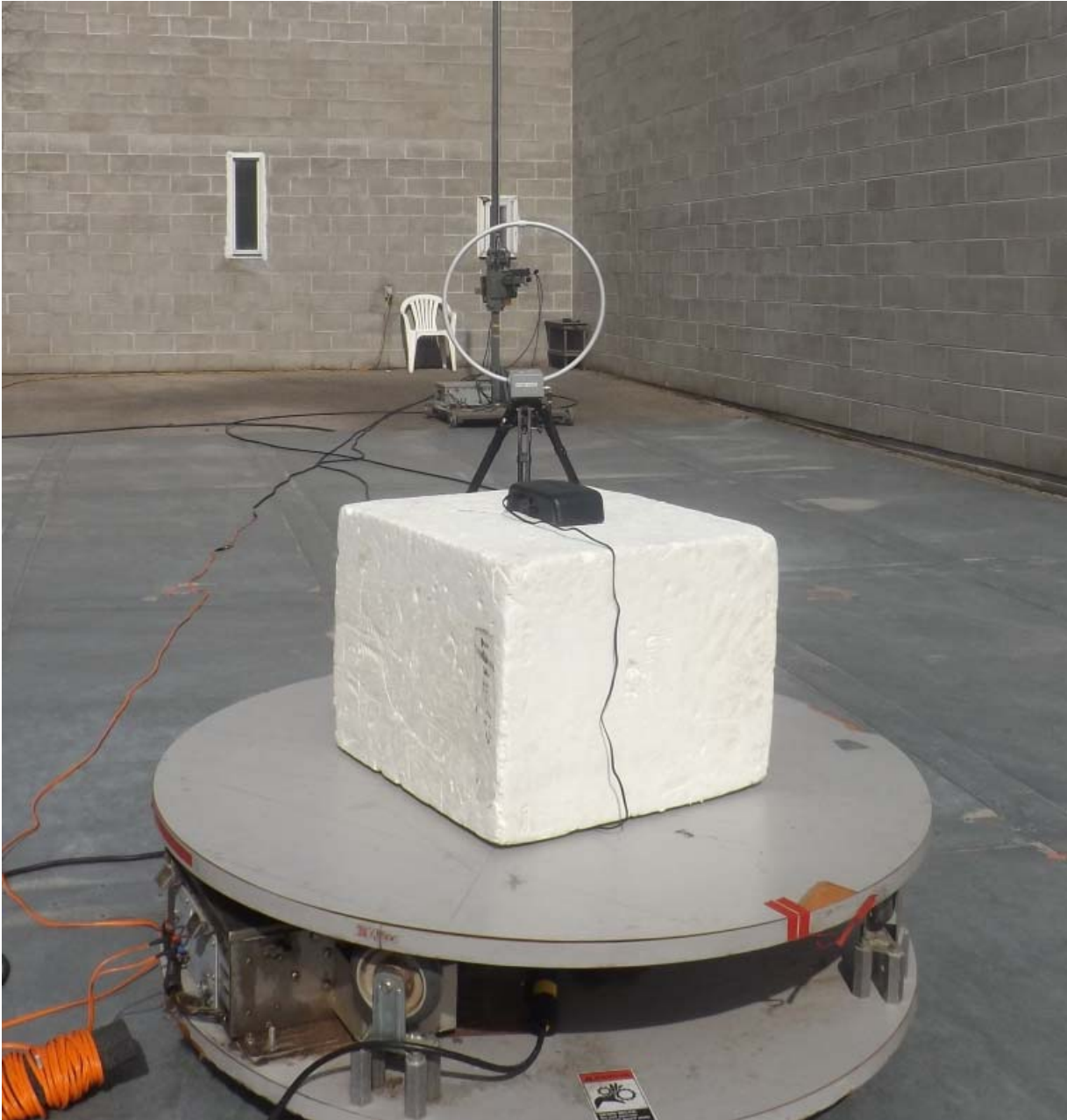
Figure E14.1 – Setup – Radiated Emissions < 30MHz, Front
