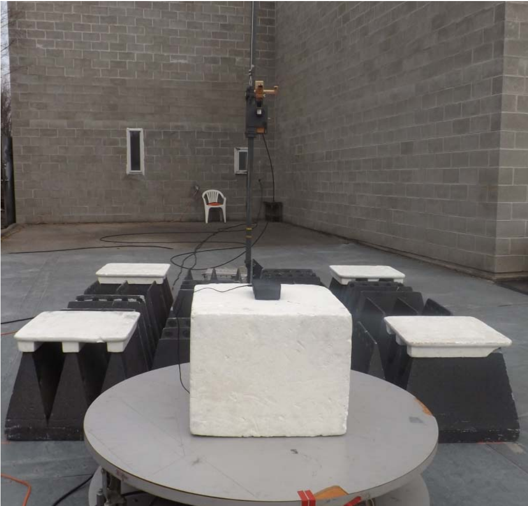
Figure E14.7 – Setup – Radiated Emissions 18 – 26.5GHz, Vertical
