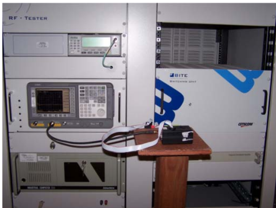
Photograph 1. Conducted Setup (RCU)
