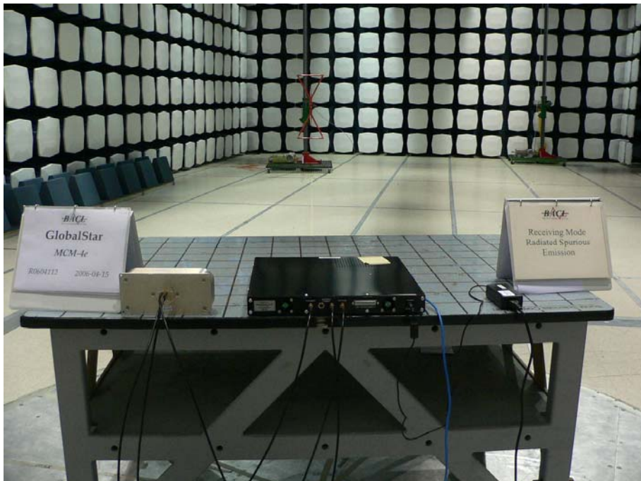
Radiated Setup – Receiver ( 10 m ) – Rear View
