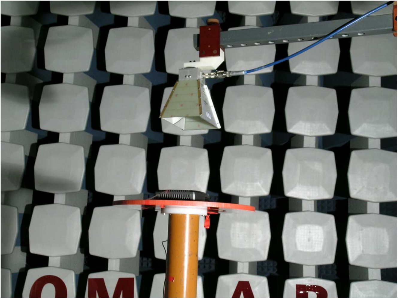
Fig 4 Test set-up when measuring electric field strength
