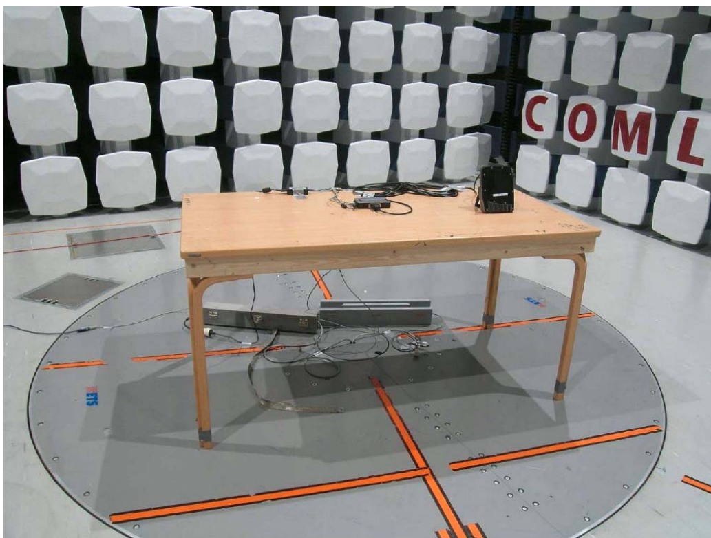
Fig 3 Test set up 1-12,75 GHz
