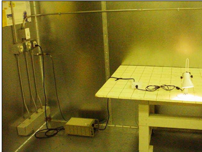
View of the EUT (“Appliance Monitor” shown) setup during emissions measurements conducted onto AC mains.
