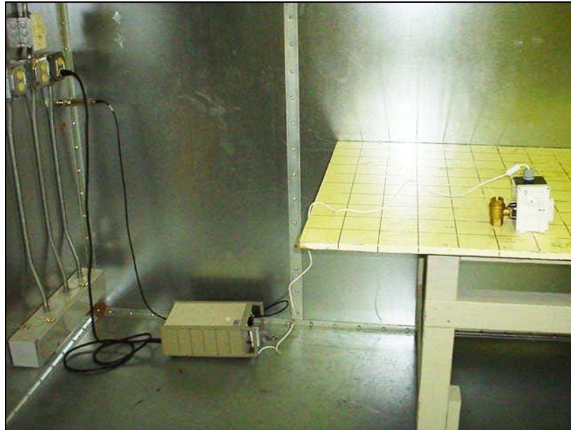
View of the EUT setup on the test pedestal, during the measurements of RF emissions onto AC Mains.
