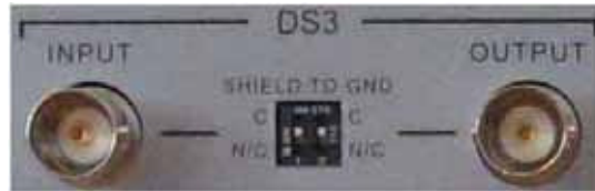
Figure 17 EX-5i-DS3 connectors and grounding switches
