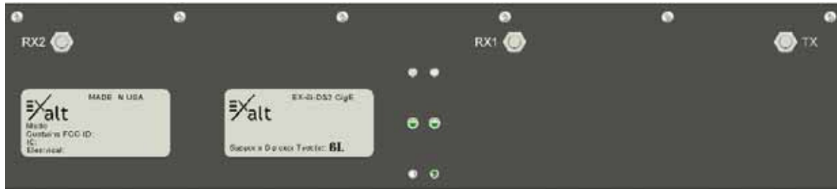
Figure 11 Rear panel without diplexers
