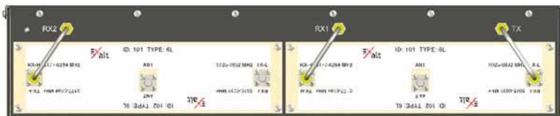
Figure 14 Typical Space Diversity diplexer configuration
