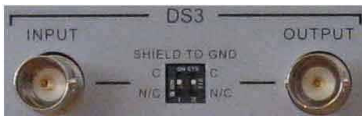
Figure 10 DS3 connectors and grounding switches
