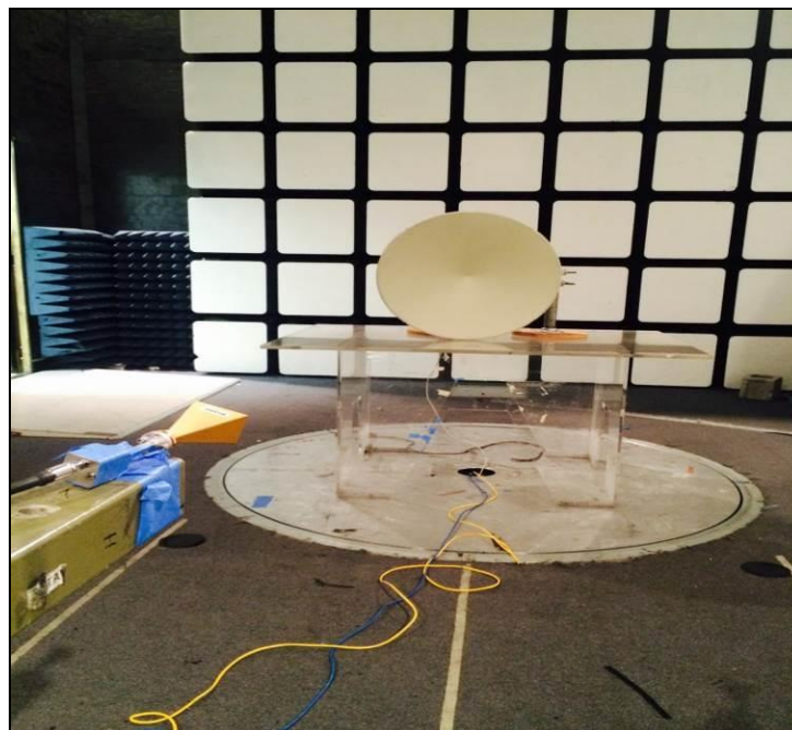
Photograph 7. Radiated Spurious Emissions, Test Setup, Above 40 GHz
