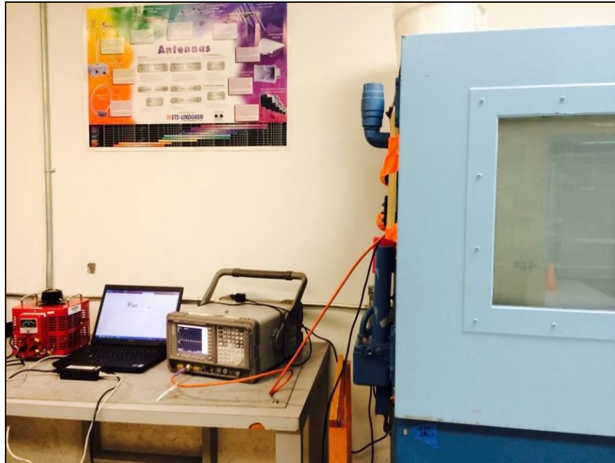
Photograph 2. Frequency Tolerance, Test Setup
