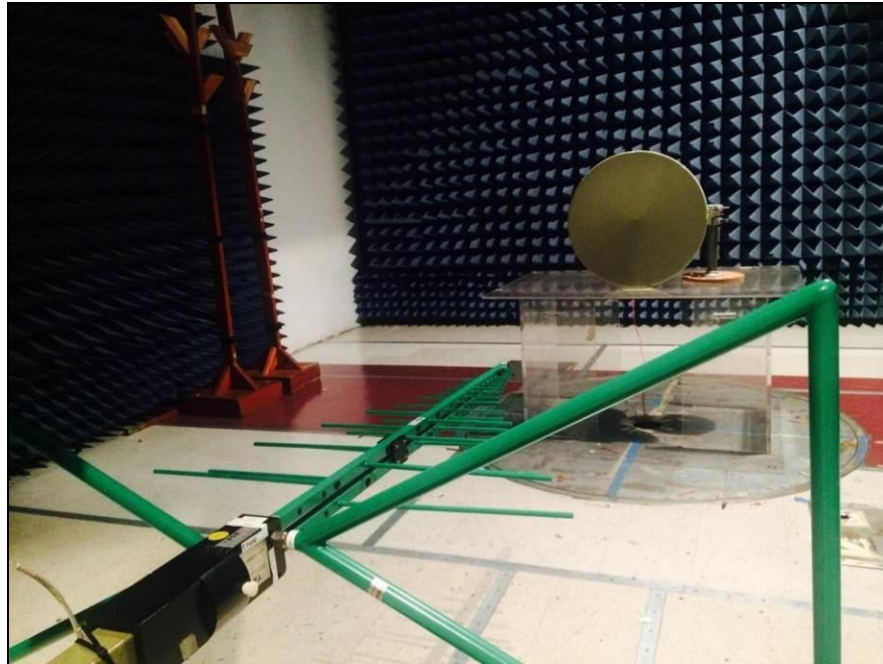
Photograph 4. Radiated Spurious Emissions, Test Setup, Below 30 MHz - 1 GHz
