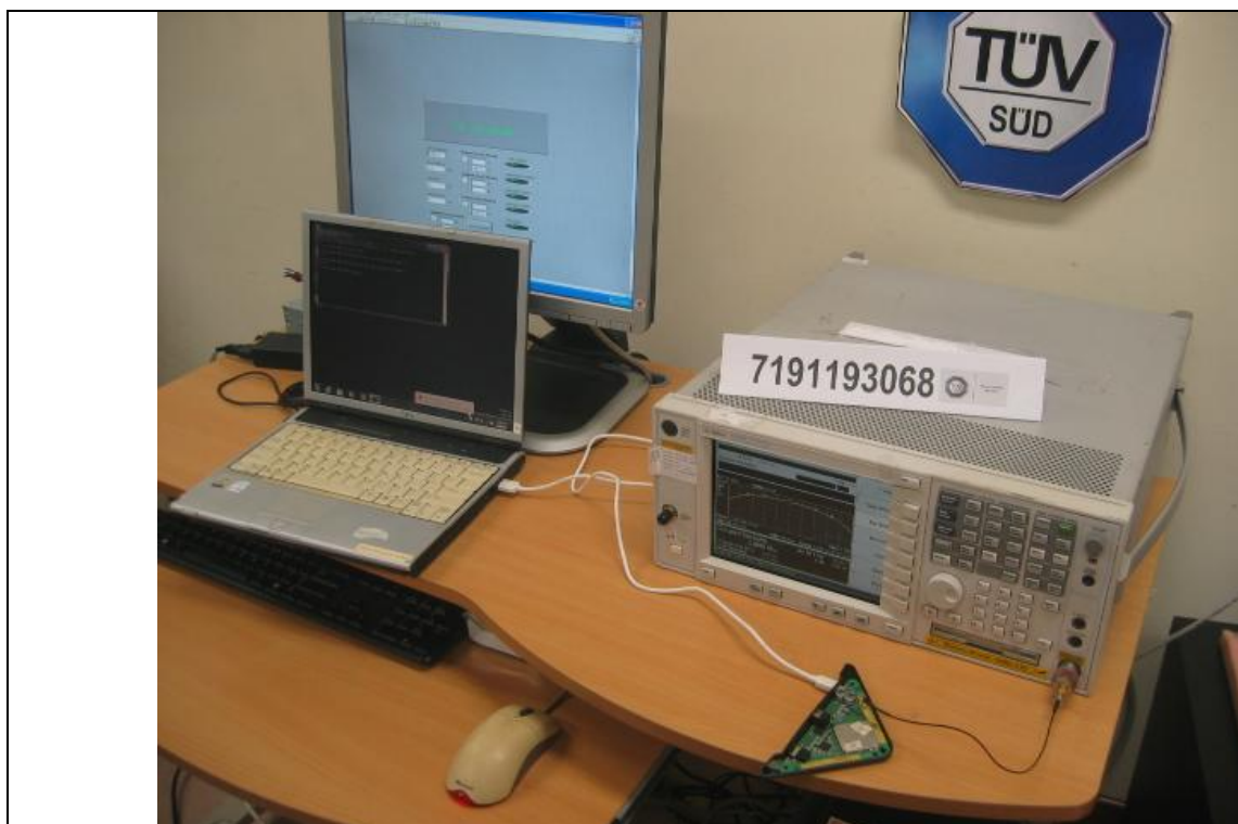
Spectrum Bandwidth (6db Bandwidth Measurement) Test Setup
