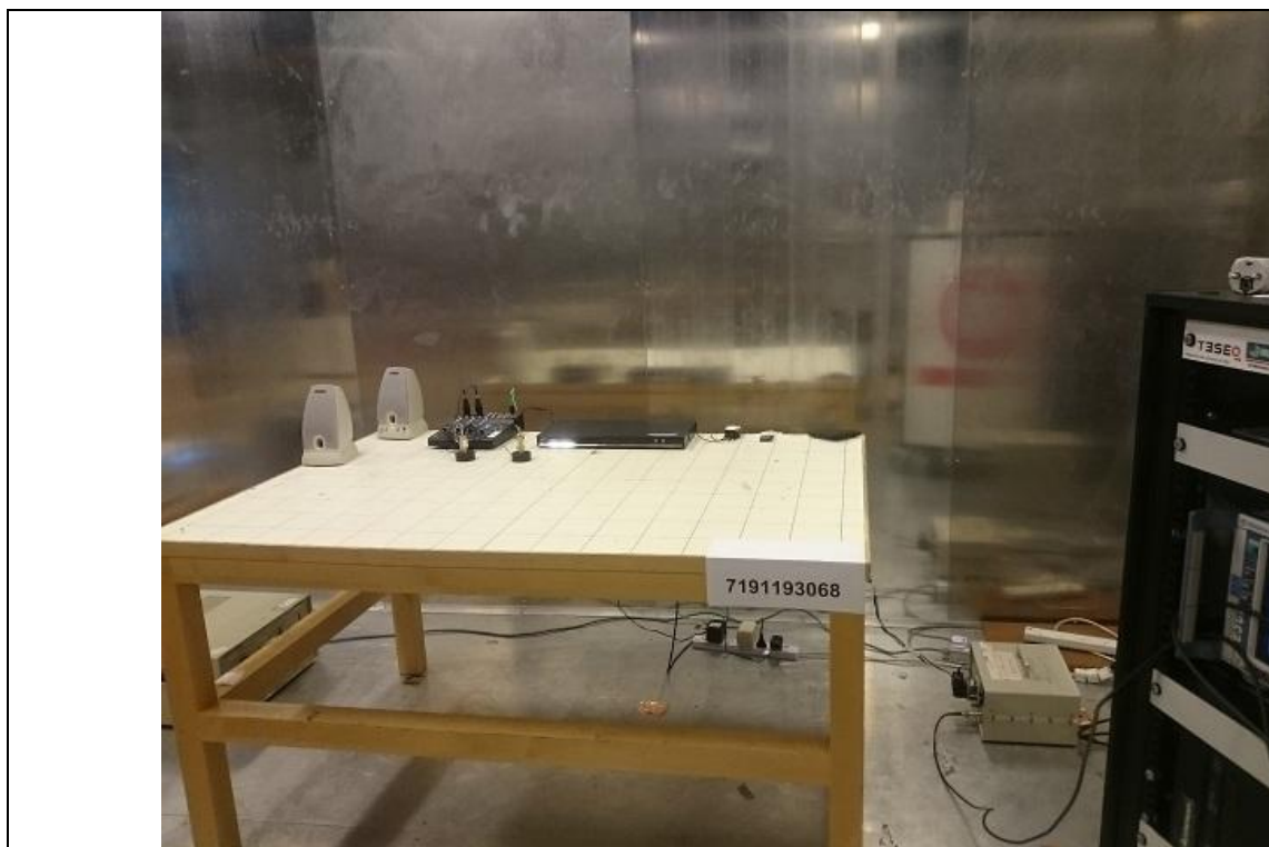
Conducted Emissions Test Setup (Front View)
