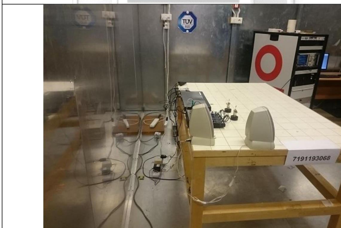
Conducted Emissions Test Setup (Rear View)
