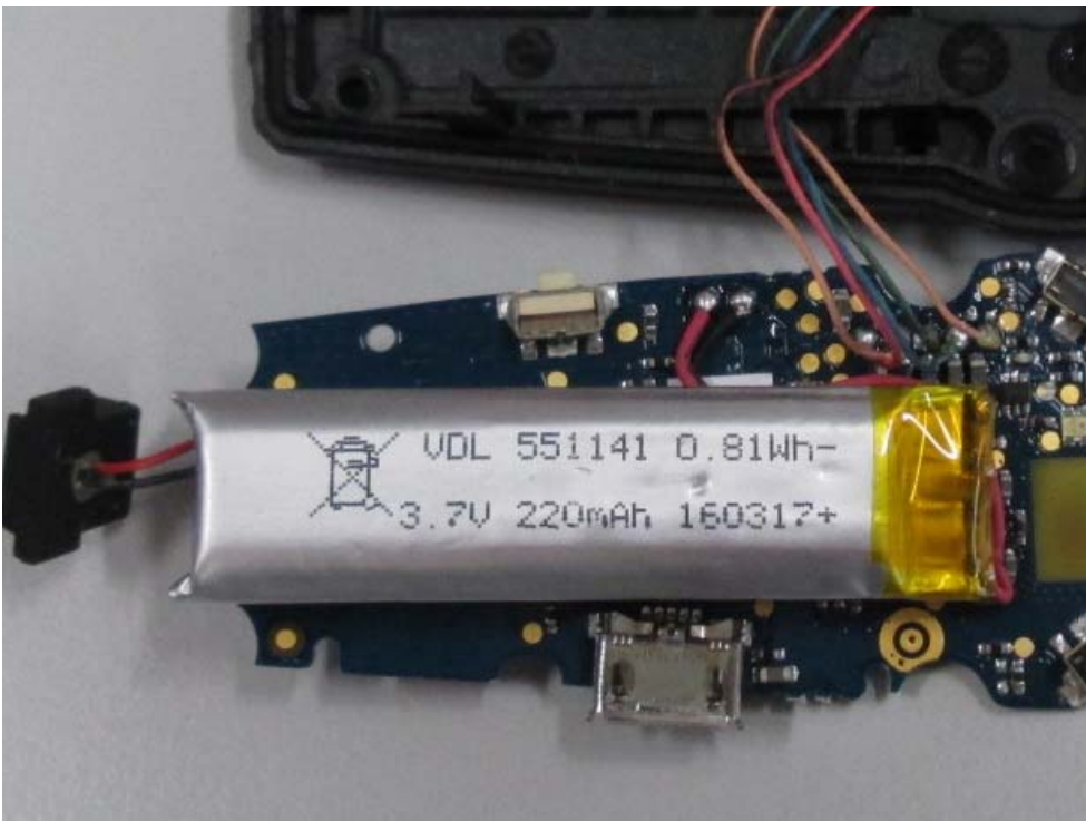
Photo A3-4: EUT #1 – Label on battery
