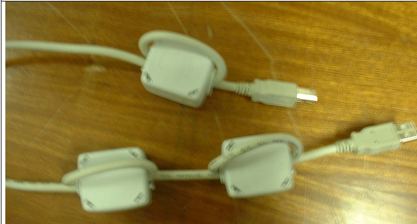
Ferrites Fitted To USB Cable
