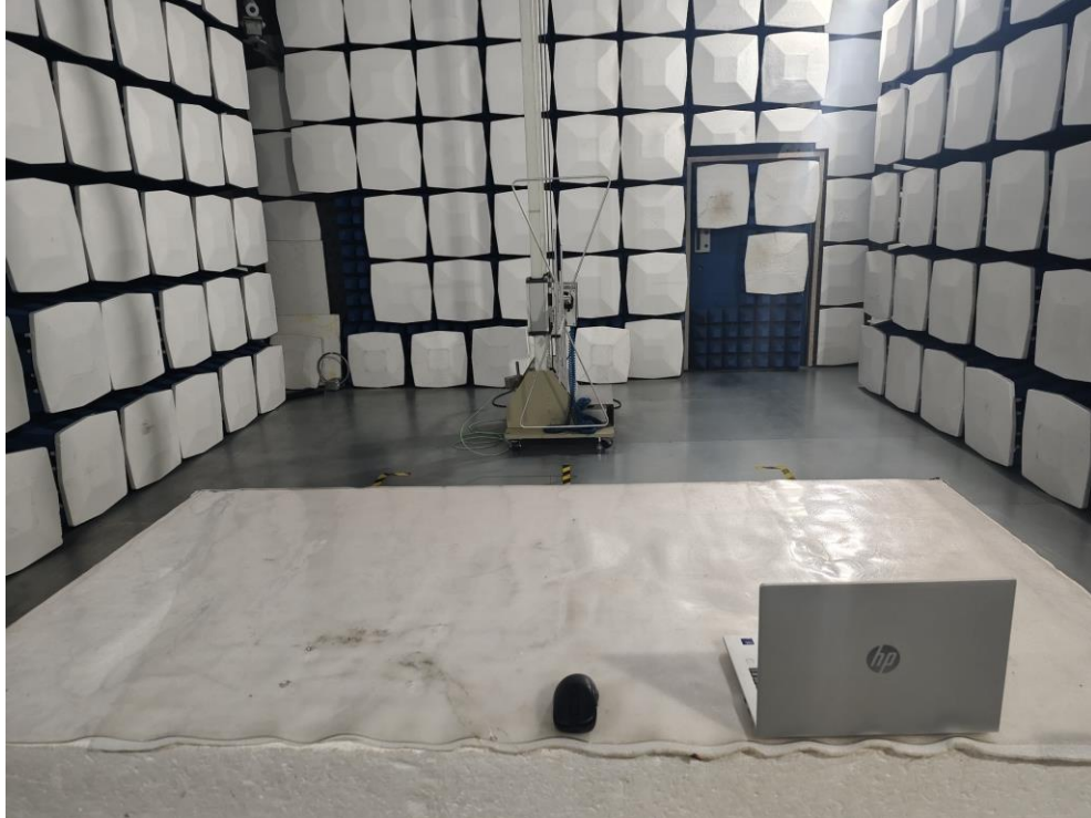
Radiated Emission Test Setup:
