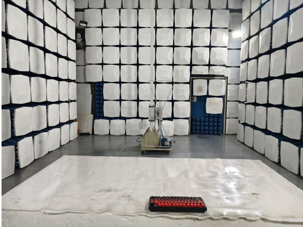
Radiated Emission Test Setup:
