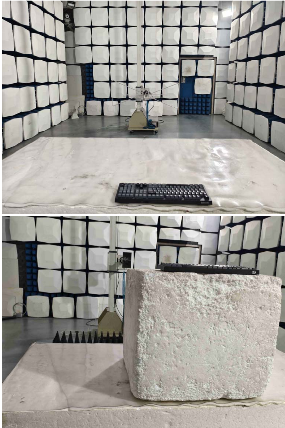
Radiated emission test view
