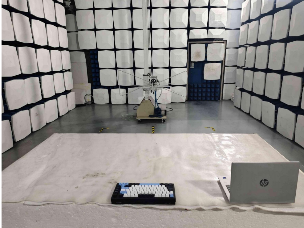
Radiated Emission Test Setup:
