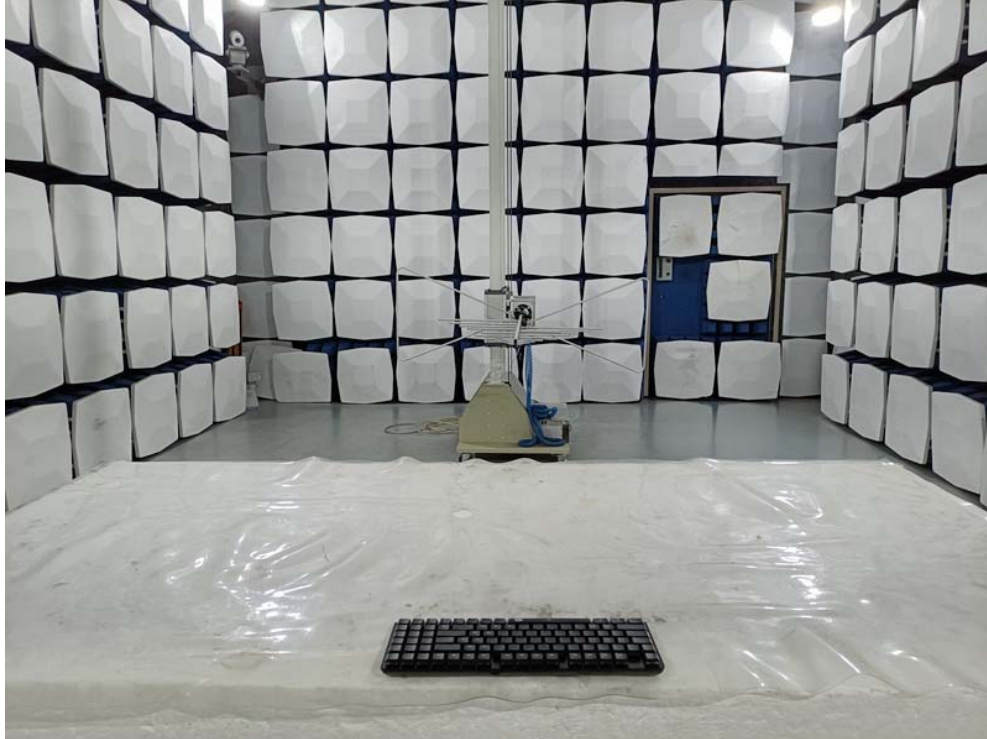
Radiated Emission Test Setup:
