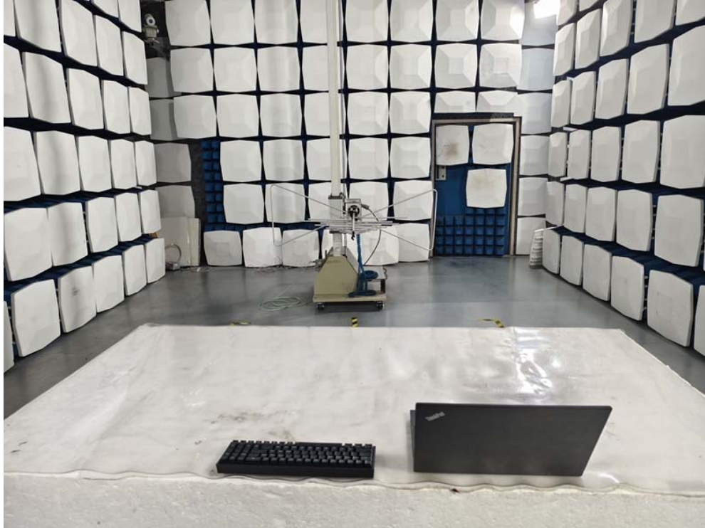
Radiated emission test view-
