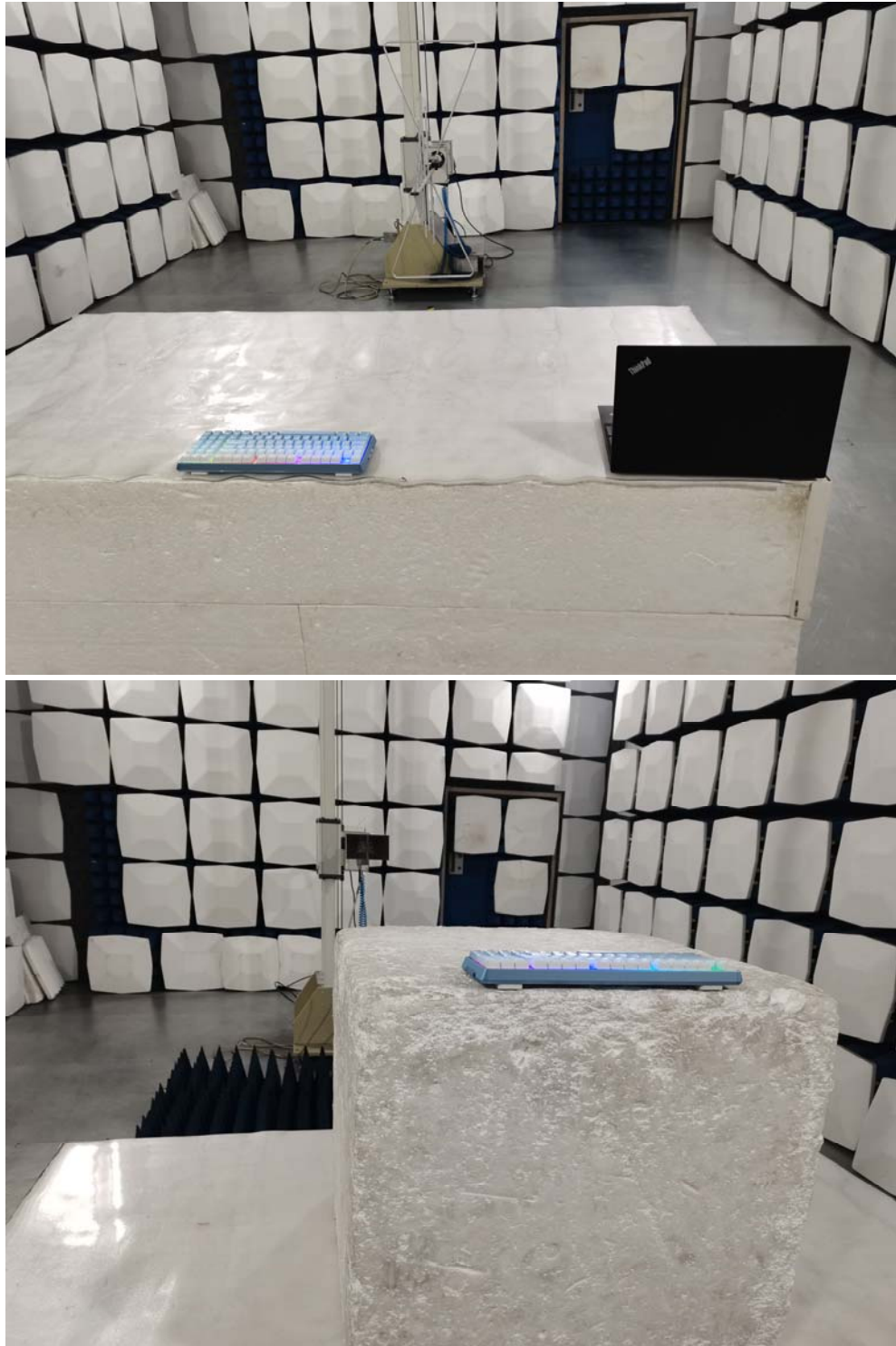
Radiated emission test view
