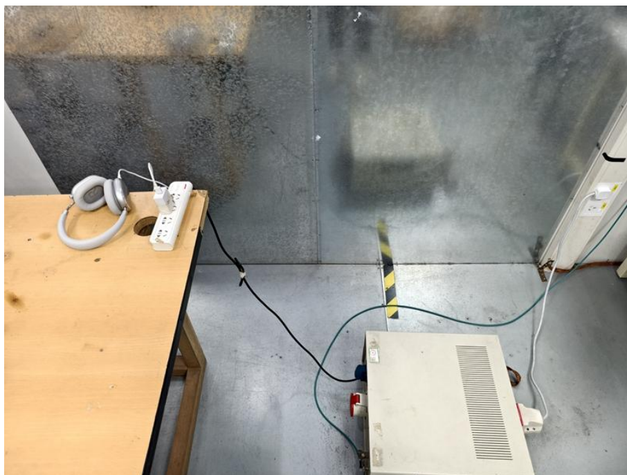
Conducted Emission Test Setup:
