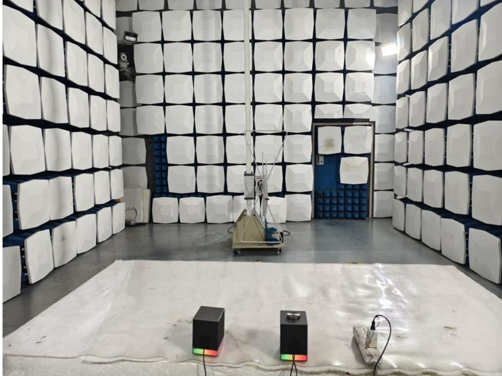
Radiated Emission Test Setup:
