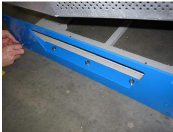
Figure 21: Caster End Plate Installation
