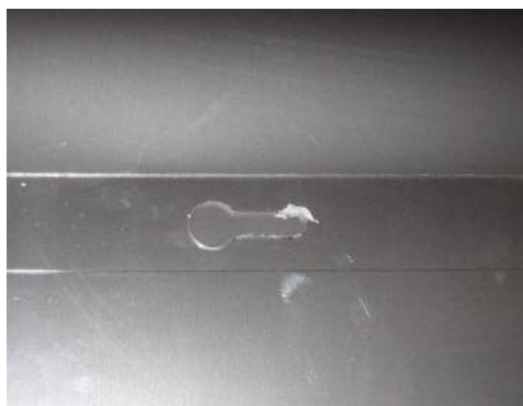
Figure 86: Inner Radome Slotted Hole and Screw Sticking Out
