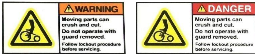
Figure 2: Belt-Drive Safety Labels
