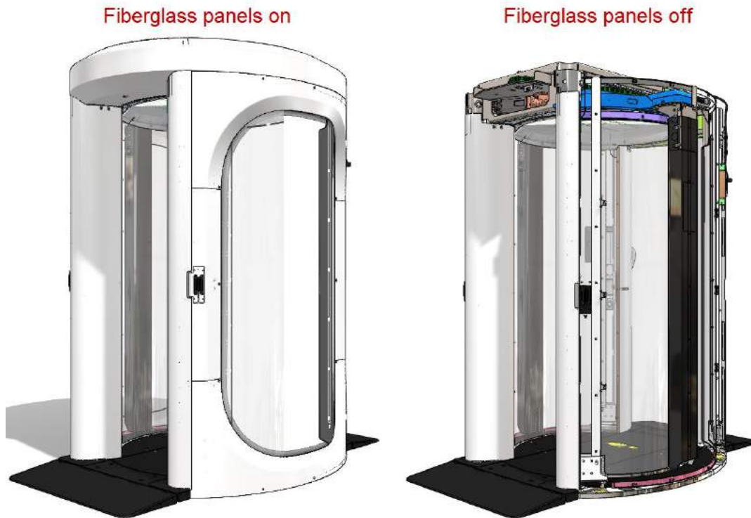
Figure 107: Fiberglass Panel Removal
