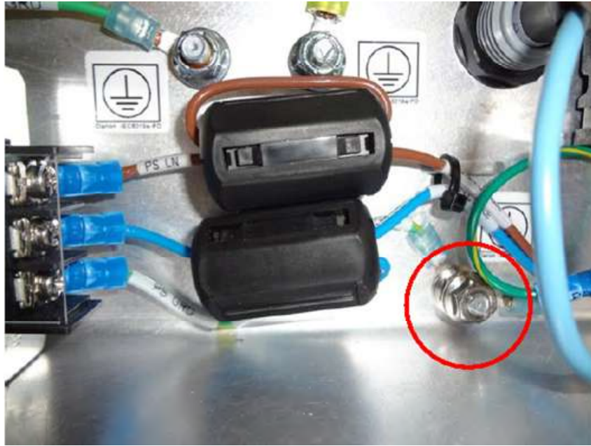
Figure 4 – Disconnect Ground Cable
