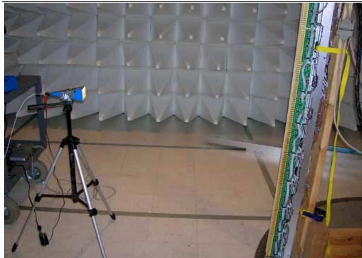
Receive Horn & Scout 100 Mast - Side View
