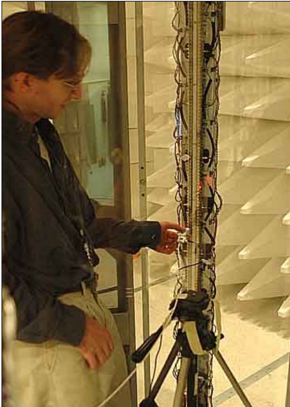
Radiated Emissions - 40-100 GHz Sample Setup Using Mixers
