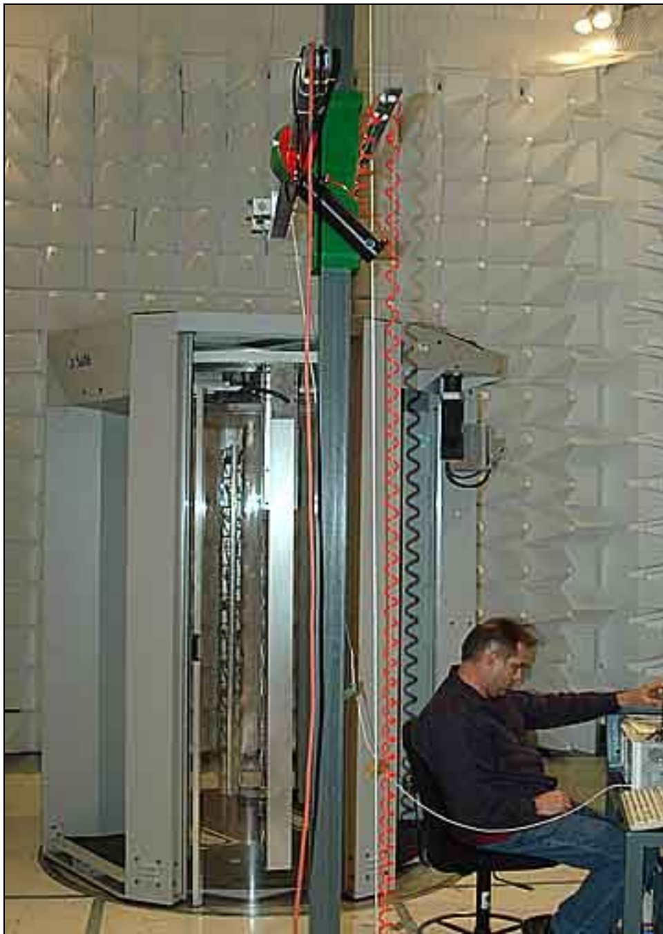
Radiated Emissions - 12-40 GHz Sample Setup at 3 Meters
