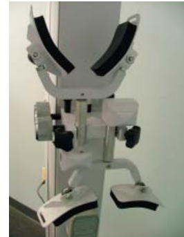
Figure 1-6. Head Braces Secured to Column
