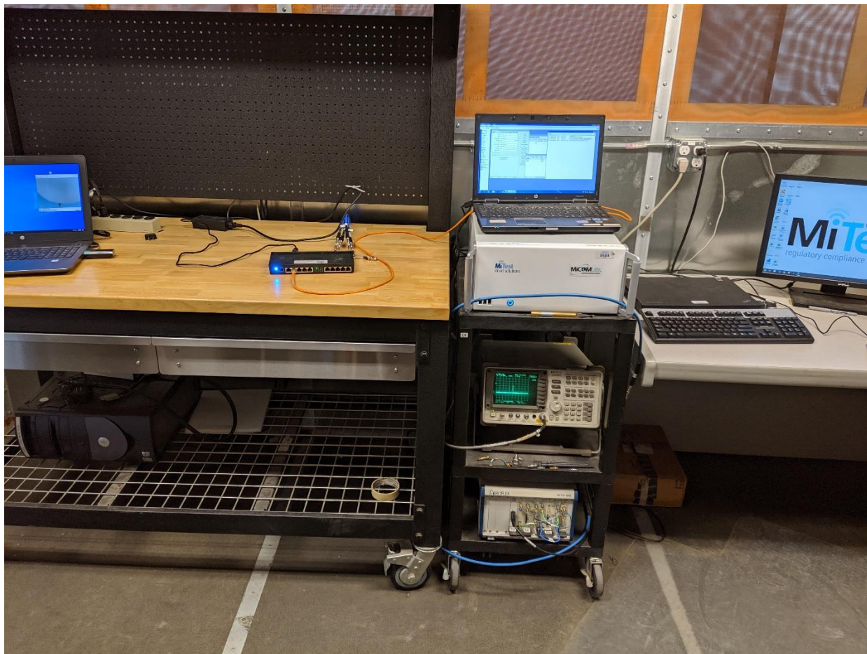
Conducted DFS Test setup
