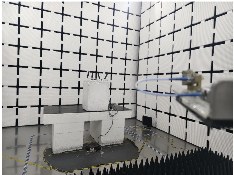
Radiation Emission Test Setup (Above 18GHz)
