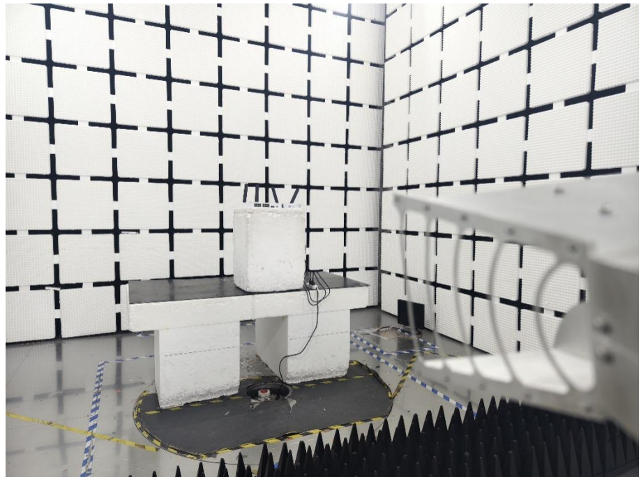
Radiation Emission Test Setup (1GHz to 18GHz)
