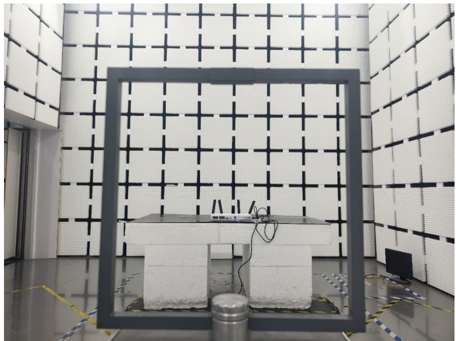
Radiation Emission Test Setup (Below 30MHz)
