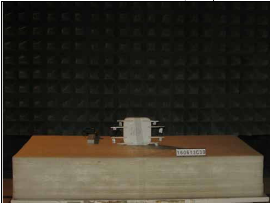
Radiated Emission Test below 1GHz (Mode C)
