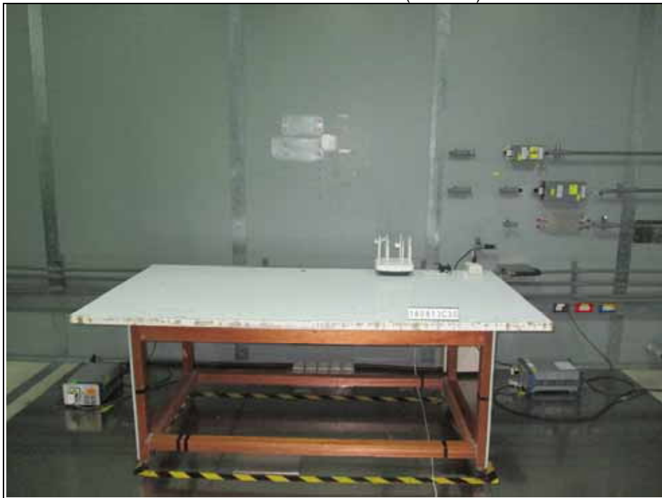
Conducted Emission Test (Mode D)
