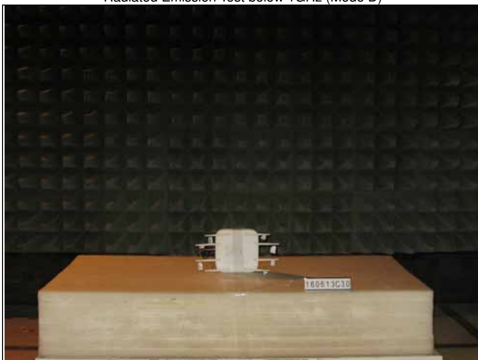
Radiated Emission Test below 1GHz (Mode D)
