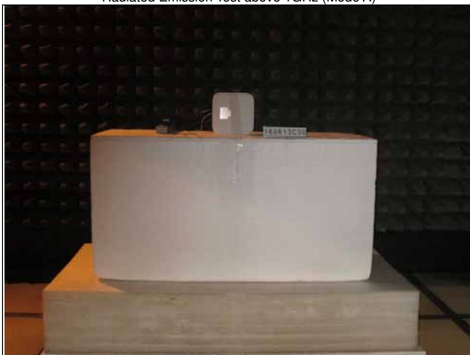
Radiated Emission Test above 1GHz (Mode A)
