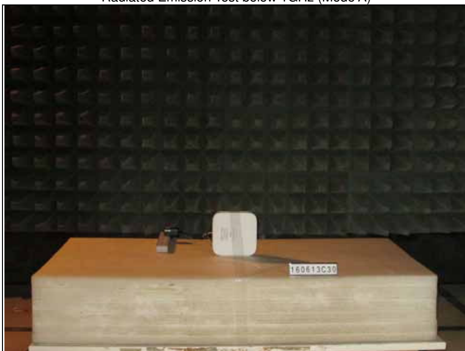
Radiated Emission Test below 1GHz (Mode A)
