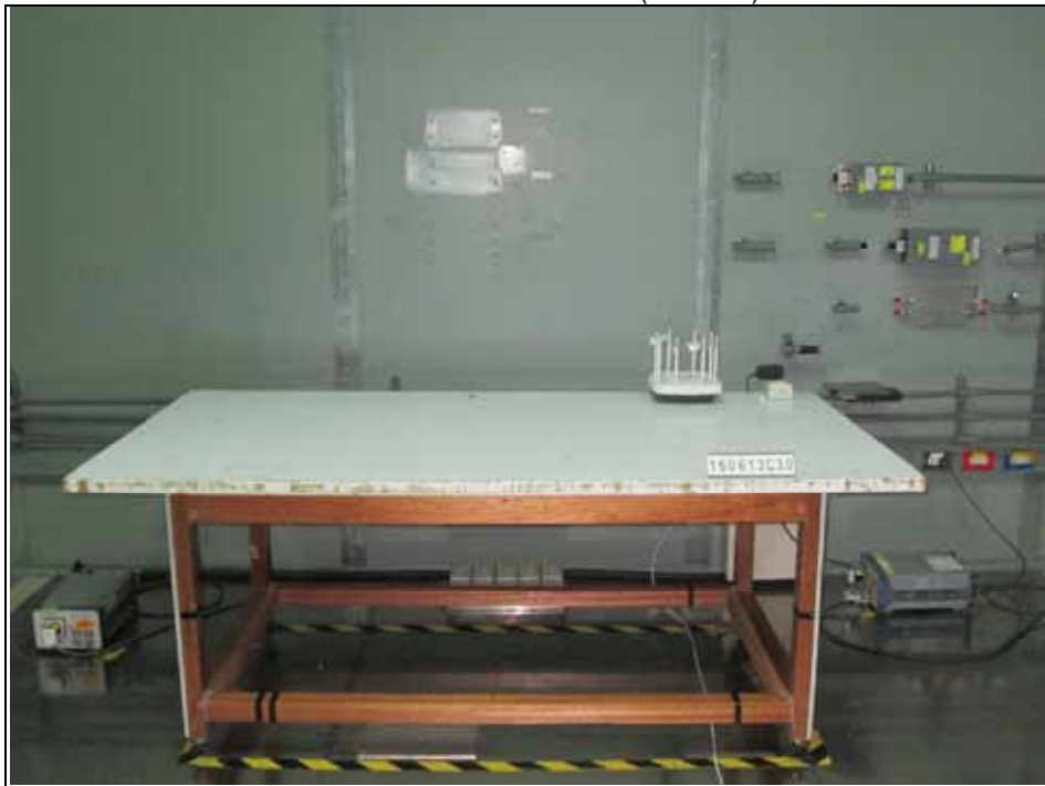
Conducted Emission Test (Mode C)
