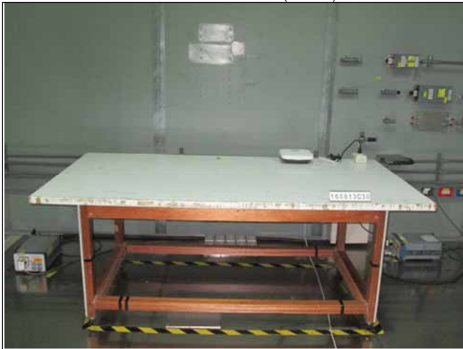
Conducted Emission Test (Mode B)
