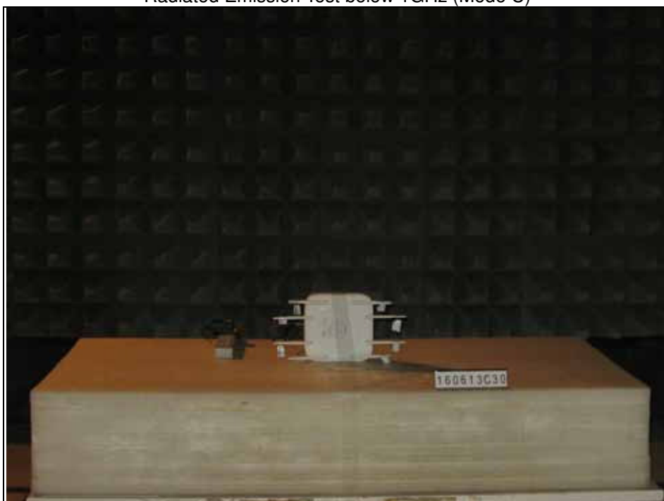
Radiated Emission Test below 1GHz (Mode C)
