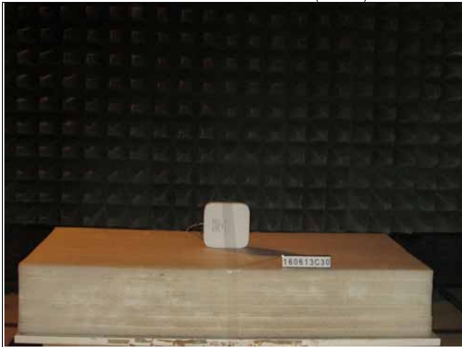
Radiated Emission Test below 1GHz (Mode B)
