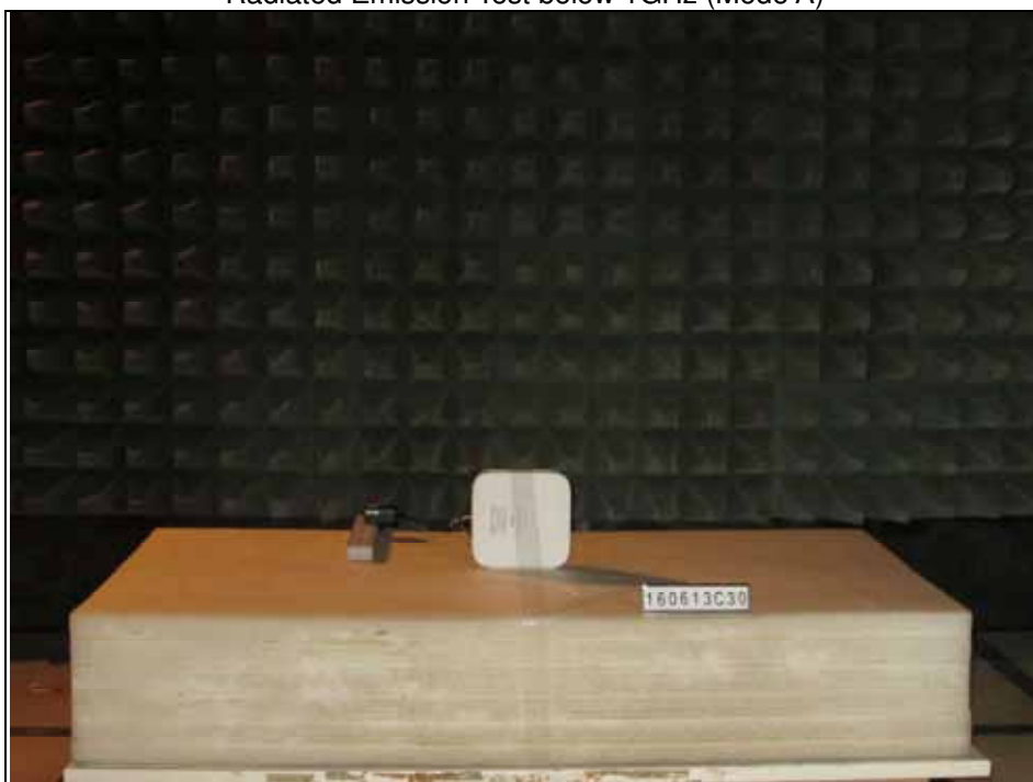
Radiated Emission Test below 1GHz (Mode A)
