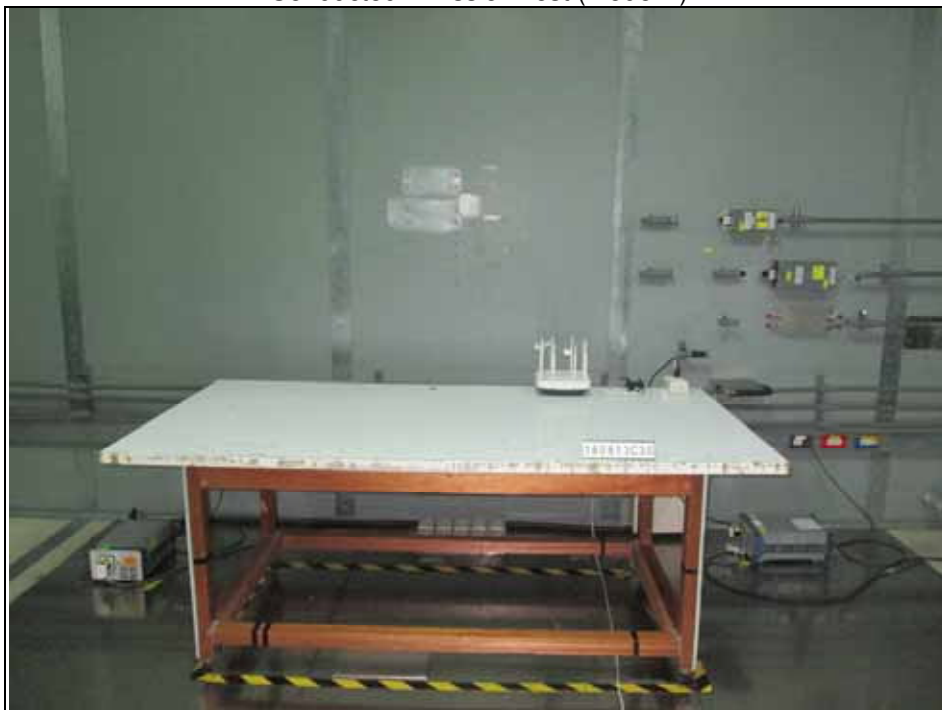
Conducted Emission Test (Mode D)
