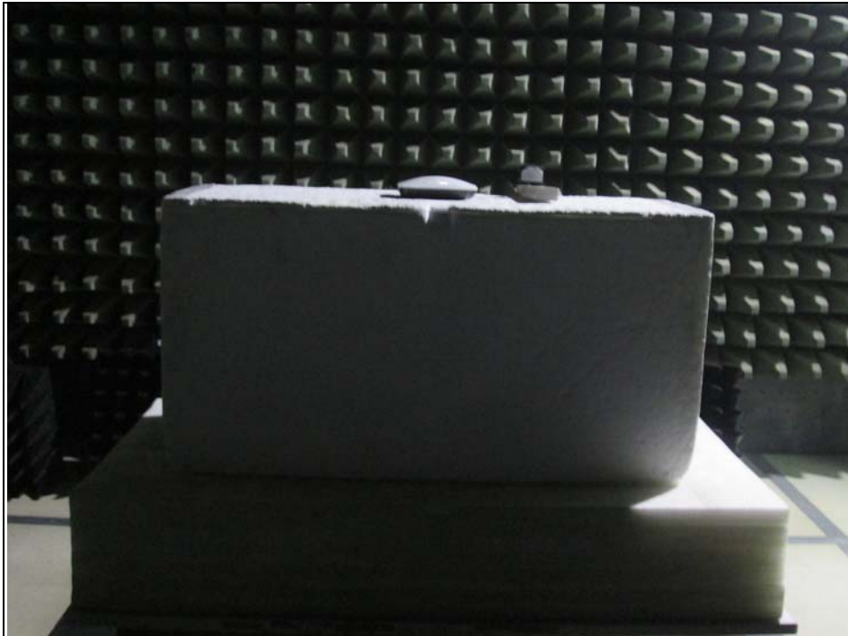
Radiated Emission Test (Above 1GHz) (X plane)
