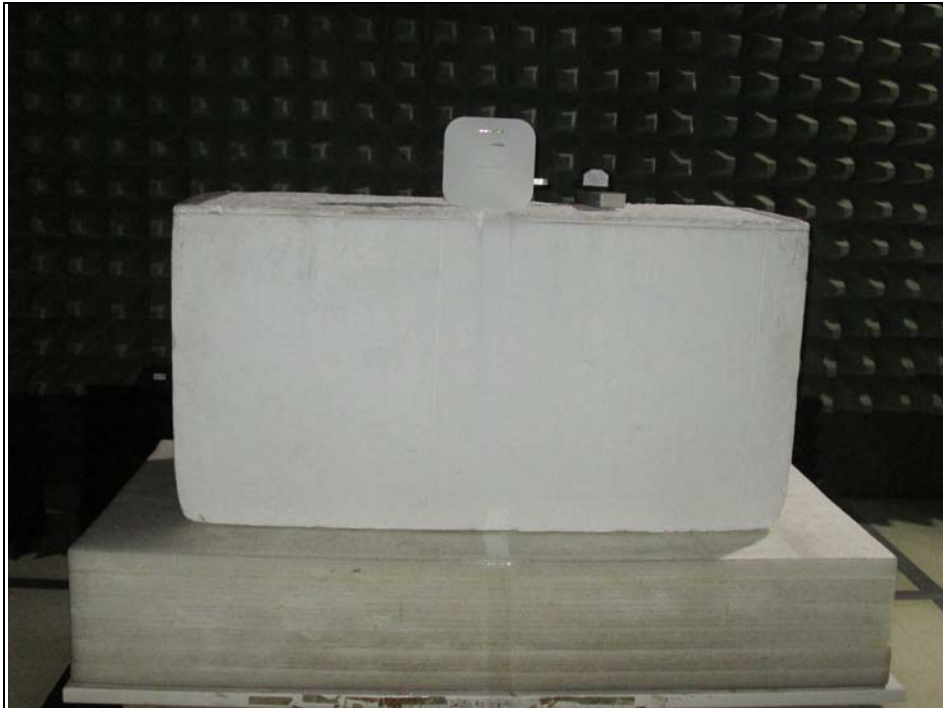
Radiated Emission Test (Above 1GHz) (Y plane)
