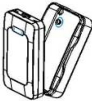
Figure 15: Removing the electronic module from the orthosis
