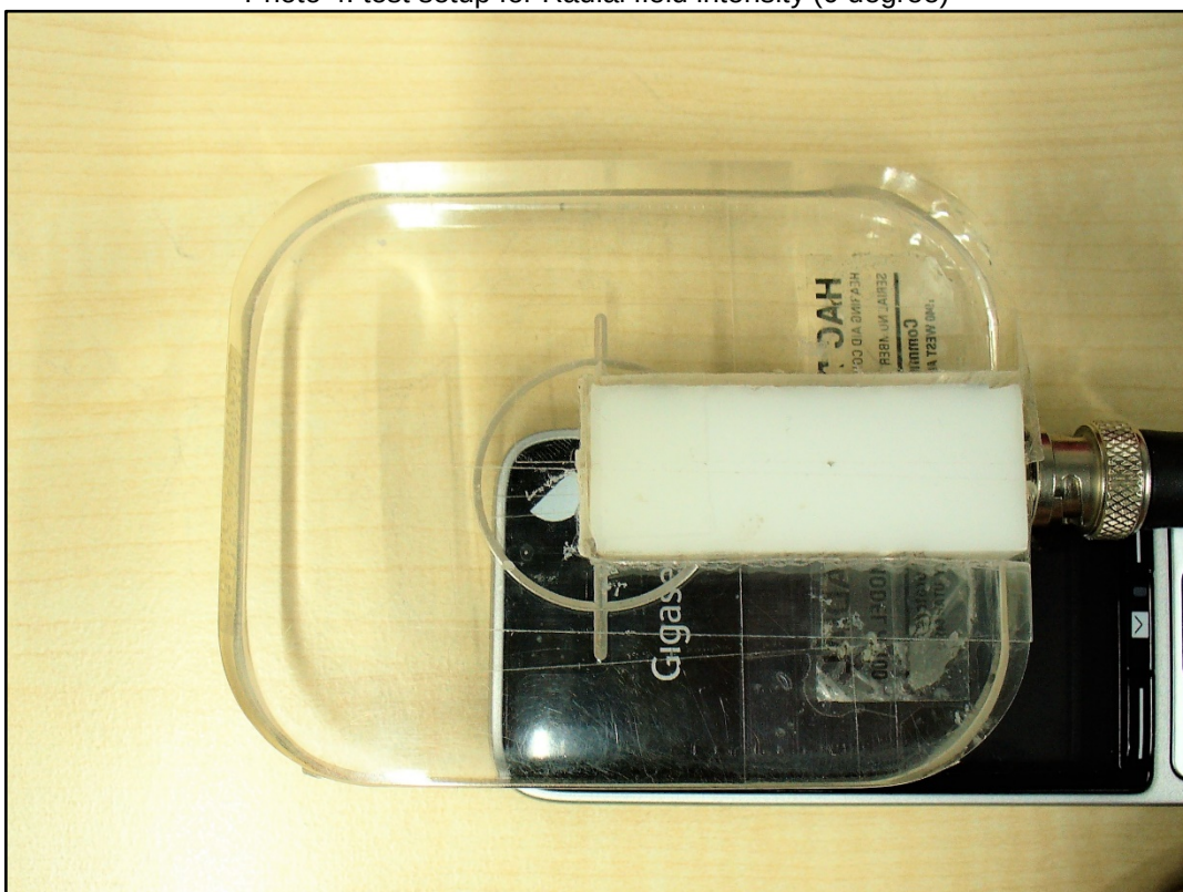
Photo 4: test setup for Radial field intensity (0 degree)
