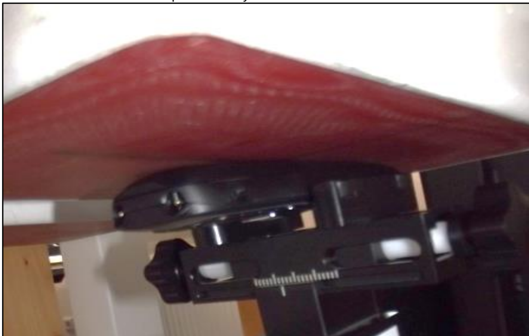
Photo 18: Test position body worn rear side with 0 mm distance
