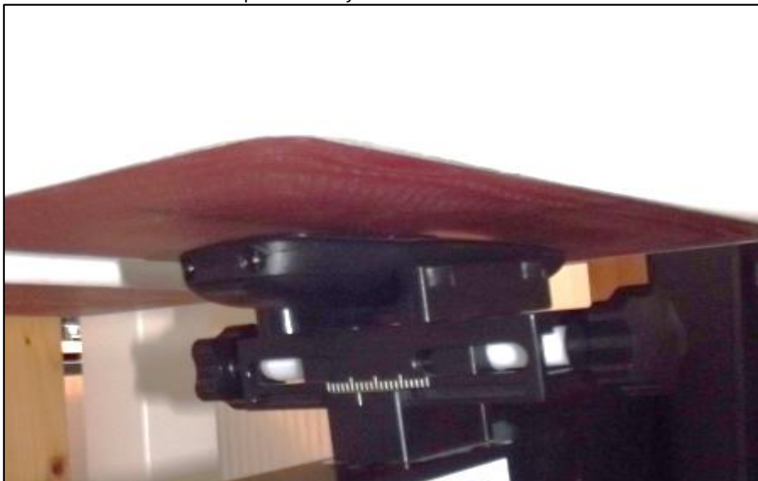
Photo 18: Test position body worn rear side with 0 mm distance
