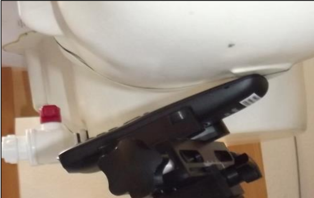
Photo 11: Test position left hand tilted 15°
