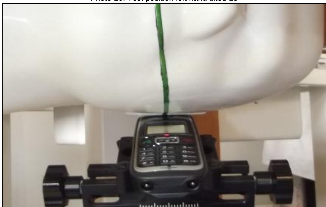
Photo 10: Test position left hand tilted 15°
