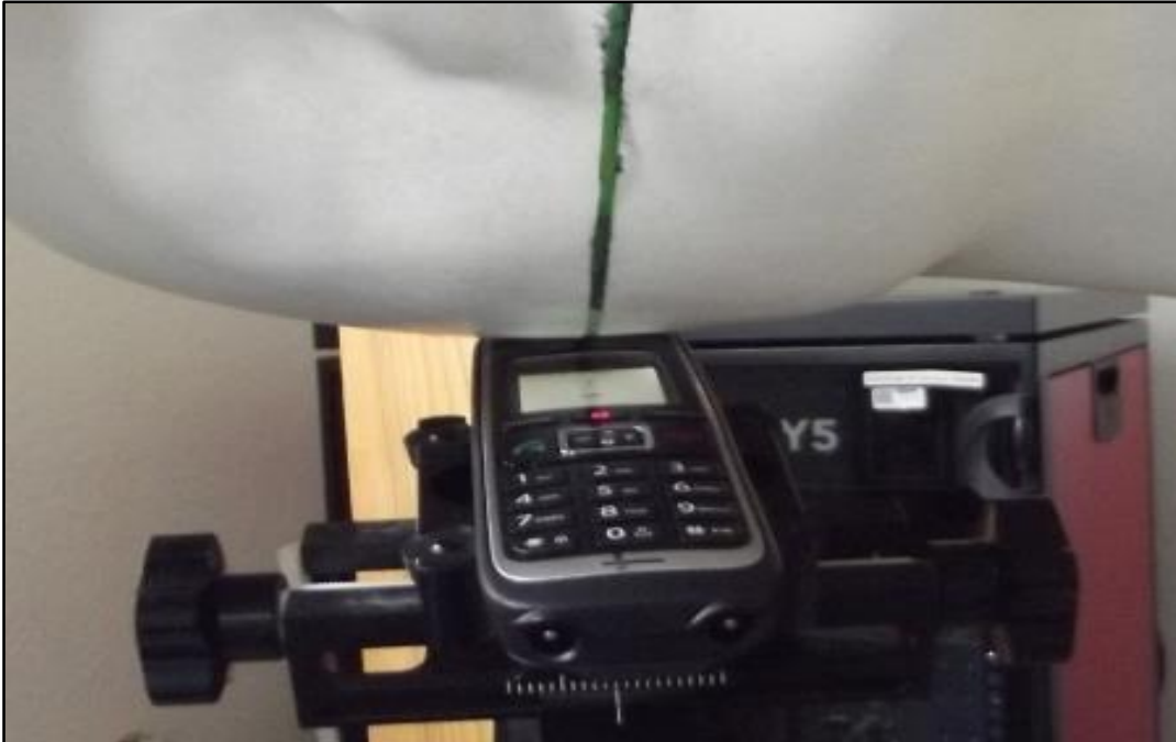
Photo 15: Test position right hand tilted 15°
