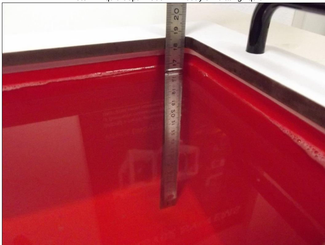
Photo 2: Liquid depth 1900 MHz body simulating liquid
