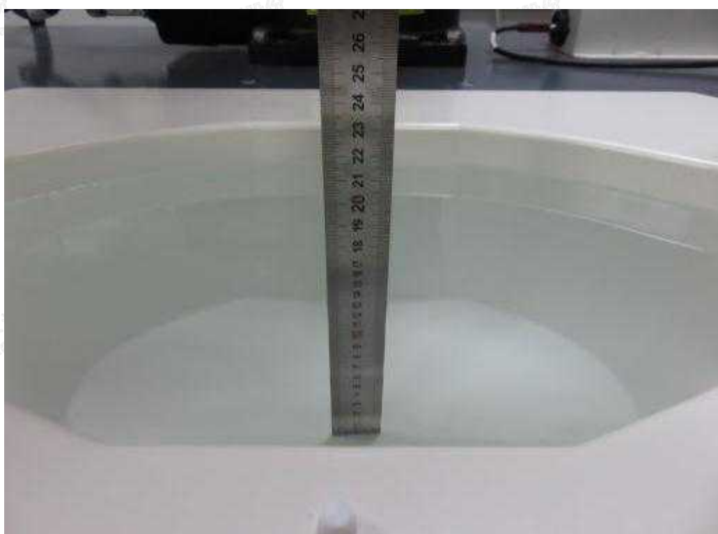
Photograph of the depth in the Body Phantom (5500MHz, 15.5cm depth)
