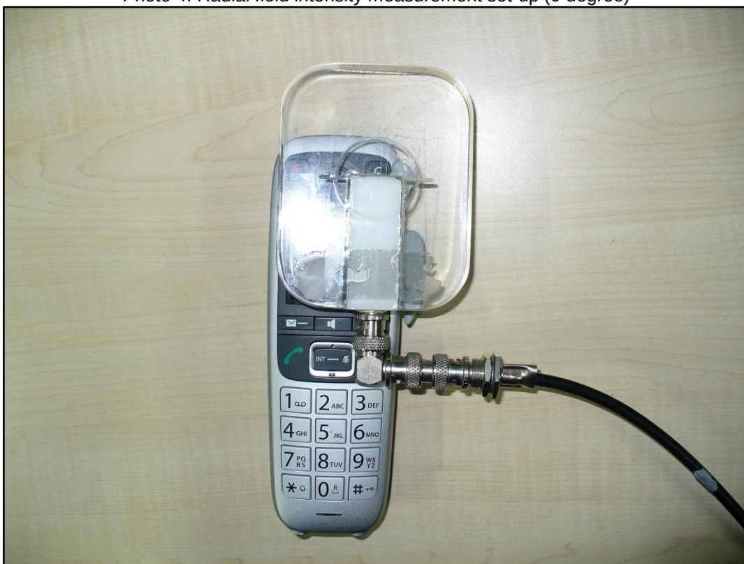
Photo 4: Radial field intensity measurement set-up (0 degree)
