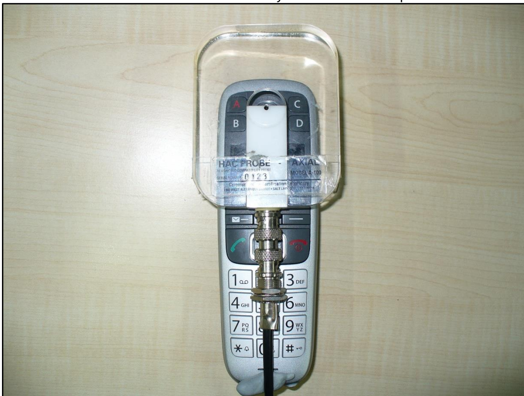
Photo 4: Radial field intensity measurement set-up (0 degree)
